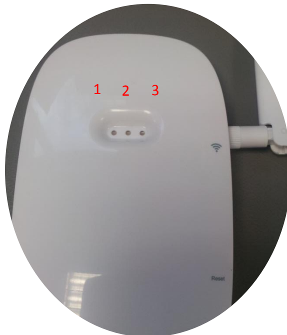
Figure 47: Maintenance check with LEDs
