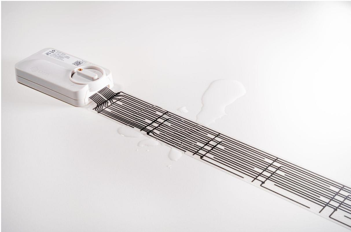
Severn WLD is LAIER's water leak detection device. The Severn WLD hardware connects to a printed sensor that is split into 12 sections or electrodes. Upon powering up with a single AA Li-SOCI<sub>2</sub> cell battery, the device connects to the LoRaWAN® network via OTAA. After running through a self-test, the device enters its run mode.
