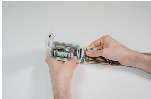
3. Close the connector by pushing down the black lever. Check that the sensor is properly connected by tugging it gently.
