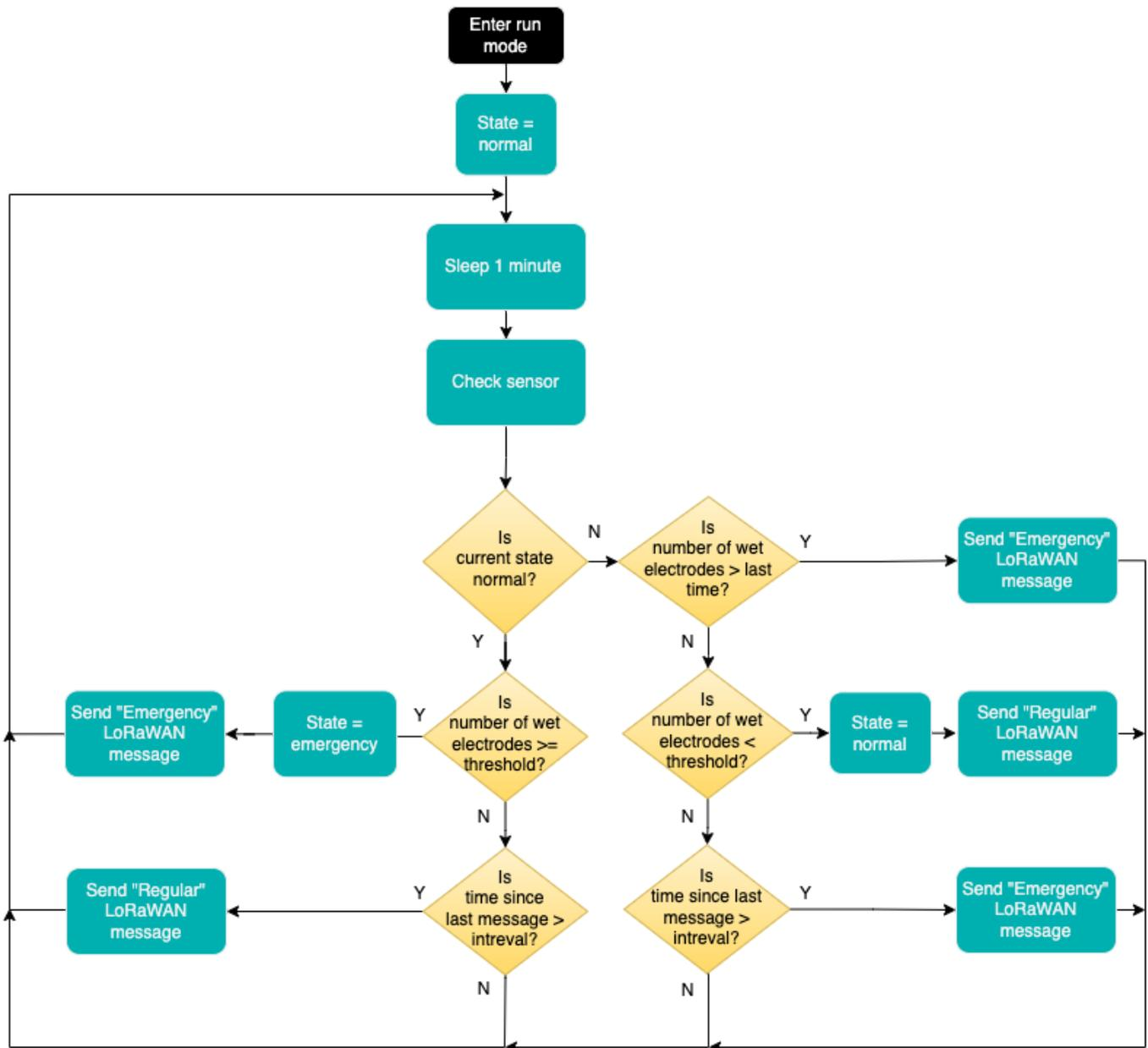
When the device enters its run mode, its state is set to normal, and it checks for the presence of water on each electrode every minute (check [Sensor Dimension and Electrode Definition](#) to see what an electrode is). By default, 4 electrodes need to be wet for the device to sense a leak.
