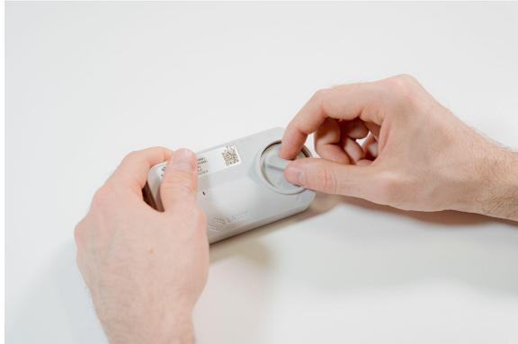
2. Open the connector, the beige part in the front of the device, by lifting the black lever of the connector upwards and insert the sensor with the print facing upwards. Insert the sensor fully, ensuring that both tabs either side of the sensor come into contact with outside of the device enclosure.
