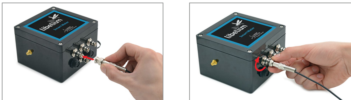
Figure: Images of the procedure to change the probes for the Smart Water Plug&Sense!
