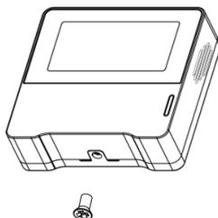
2. Paste 3M double-sided tape to the back of the device, then tear the other side and place it on a flat surface.
