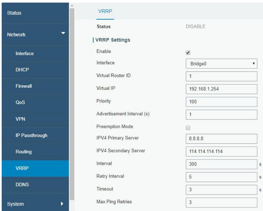
The screenshot shows the VRRP configuration page. The left sidebar has a menu with the following items: Status, Network, Interface, DHCP, Firewall, QoS, VPN, IP Passthrough, Routing, VRRP (selected), DDNS, and System. The main content area is titled VRRP and shows the following configuration:
