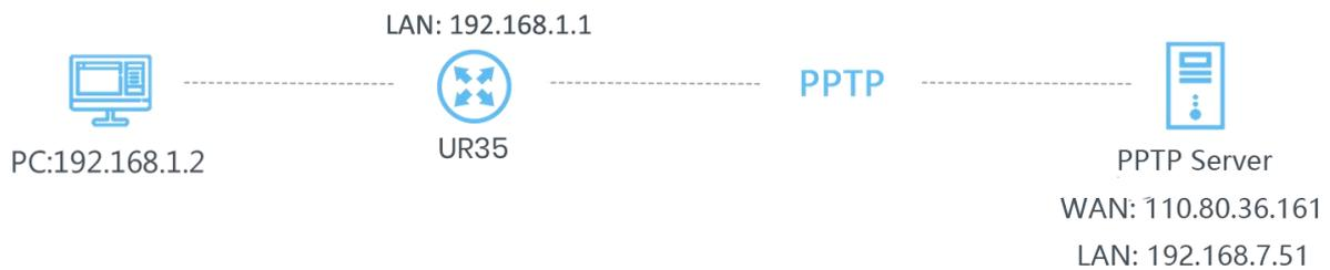
Configure the UR35 as PPTP client to connect to a PPTP server in order to have data transferred securely. Refer to the following topological graph.
