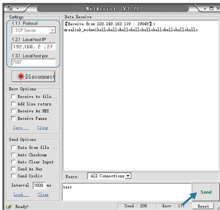
8. After serial communication test is done, you can connect PLC to RS232 port of the UR35 for test.
