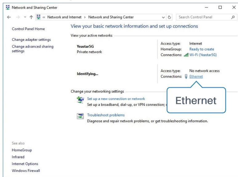
2. Go to "Properties" → "Internet Protocol Version 4(TCP/IPv4) ", select "Obtain an IP address automatically" or "Use the following IP address", then assign a static IP manually within the same subnet of the device.
