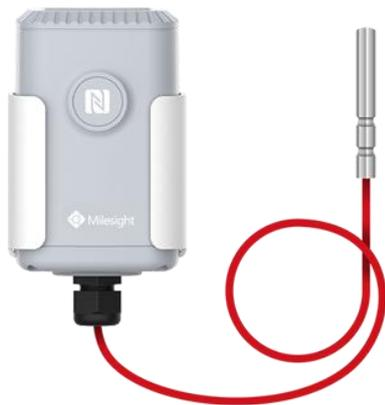
EM500-PT100 resistance temperature sensor is designed for measuring wide range of temperature in harsh environments and transmitting data using LoRaWAN<sup>®</sup> technology. With this low power consumption technology, EM500-PT100 can work up to 10 years with 19000 mAh battery. Combining with Milesight LoRaWAN<sup>®</sup> gateway and Milesight IoT Cloud solution, users can manage all sensor data remotely and visually.
