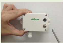
2. When the temperature and humidity detected by R718AB is compared with the last reported values, when the temperature change is exceeded 1°C (default) or the humidity change is exceeded 1%(default),it will report current values.
