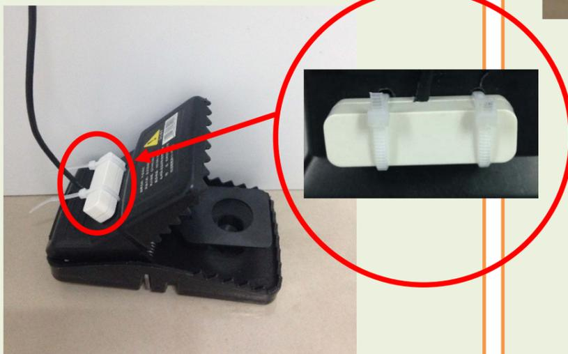
3. The figure shows the vibration sensor (R718DA)
