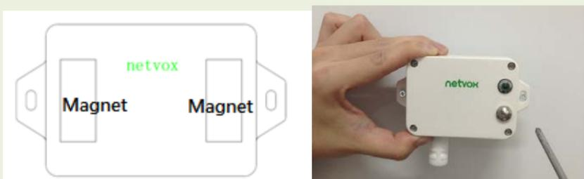
2. Tear off the 3M glue at the bottom of the reed switch probe and the magnet (as the red frame in the figure above). Then, stick the reed switch probe to the door and is parallel to the magnet (as the figure on the right).
