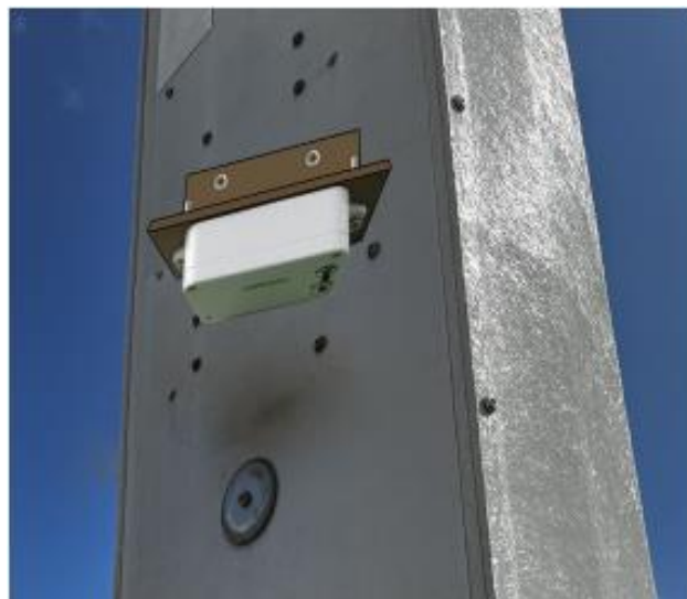
Figure 1. Install the R720E upside down
