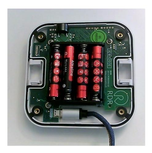
The device is a so called USB slave that emulates a serial port over its USB socket. Windows 10 should automatically install a Virtual-Com-Port Driver (VCP).
