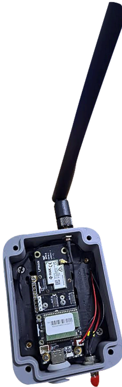
Figure 2: WisMesh WiFi MQTT Gateway in the Unify Enclosure 100x75x38mm
