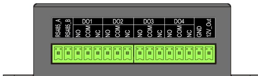
Figure 2: RAK2461 WisNode Bridge IO Lite interfaces bottom (RS485-DOx4)
