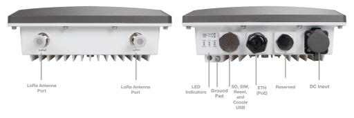
Figure 3: RAK7289V2/RAK7289CV2 Interfaces
