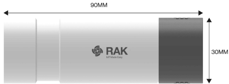
Figure 1: RAK2560 WisNode Sensor Probe dimensions
