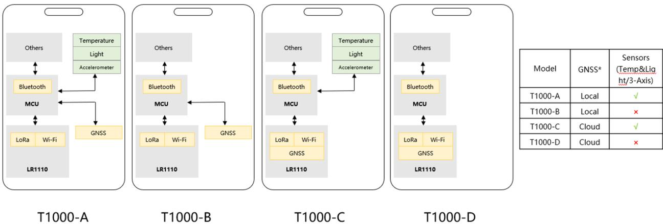
The main chip used in the T1000 is based on [Semtech LR1110](#), LR1110 has built-in GNSS function to obtain encrypted satellite data, which is finally uploaded to the Cloud and parsed by LoRa Cloud.
