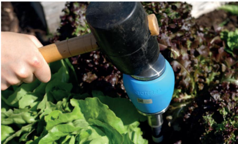
*Hammer the sensor into the ground*
