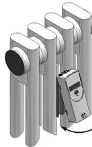
As soon as the heat cost allocator is fixed to the aluminium rail, the display will show the following message:
