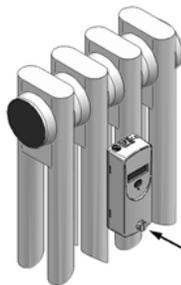
Now the heat cost allocator can only be opened by destroying the seal.
