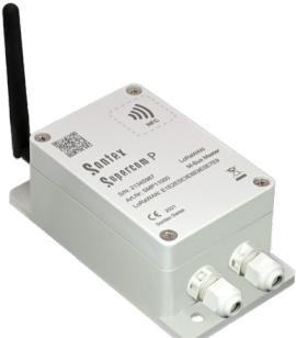
The Supercom P Pulse-Radio Converter is a combined converter for remote reading of all types of consumer devices with digital pulse output. It also has a wired M-Bus master with which up to two slaves can be connected. The Supercom P stores the consumption values and transmits the data via the LoRaWAN® network. The pulse-radio converter is programmable, so backflow and/or manipulation detection can be set.
