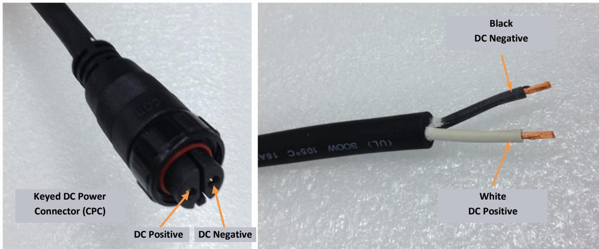
Figure 6: Direct DC Power CPC Connector Connection Polarity
