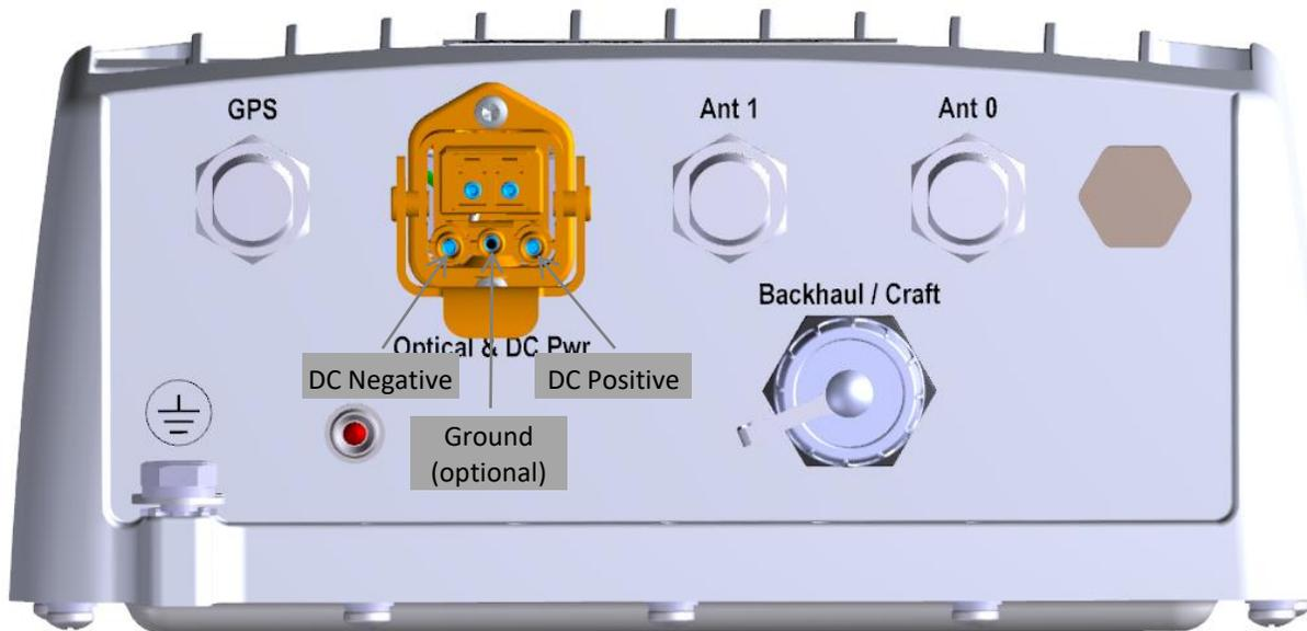
**Figure 16: Hybrid Connector Direct DC Power Connection Polarity**
