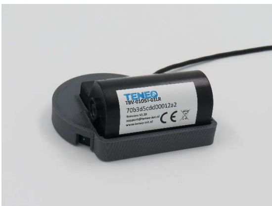
Figure 6: Sensor fill level on a charging pad (incl. 3D printed attachment).
