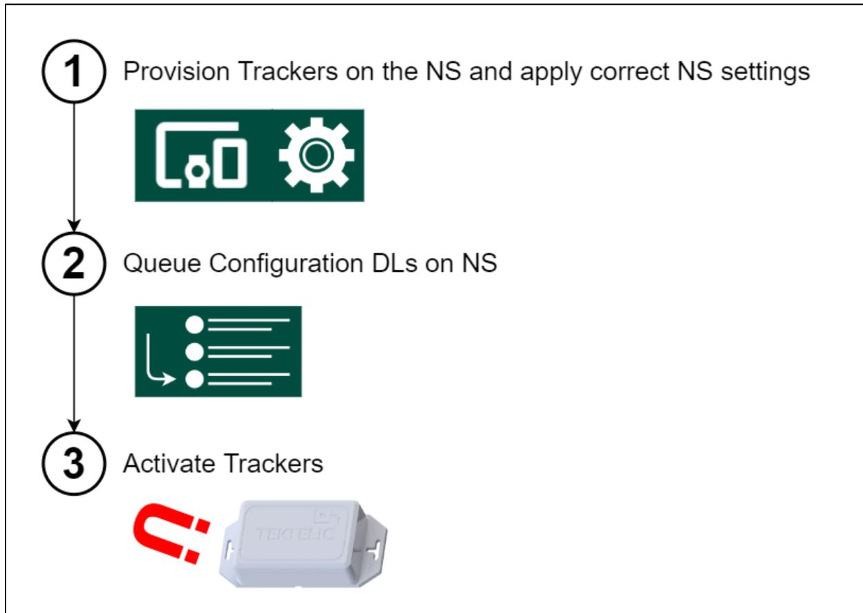
**Figure 1: High-Level Activation & Configuration Procedure**
