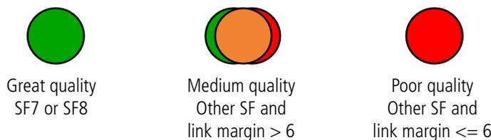
The result of the test is given by the devices after around 20 seconds following the Join Accept. It is visible through the sole thanks to the LED. With this information the installer know the quality of the network and can move the product to a place with a better coverage.
