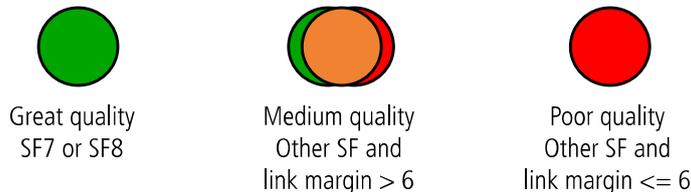
The result of the test is given by the devices after around 20 seconds following the Join Accept. It is visible through the sole thanks to the LED. With this information the installer know the quality of the network and can move the product to a place with a better coverage.
