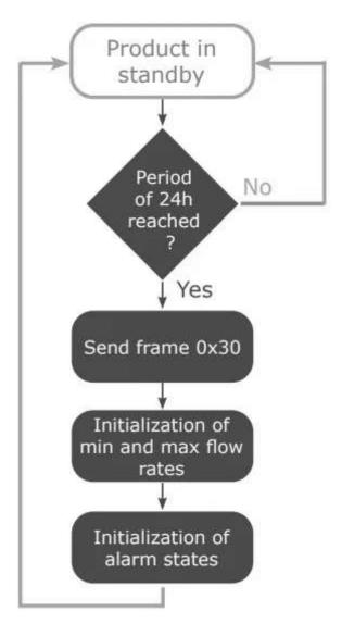
The transmission period of the daily frame is fixed (24 hours) and not configurable.
