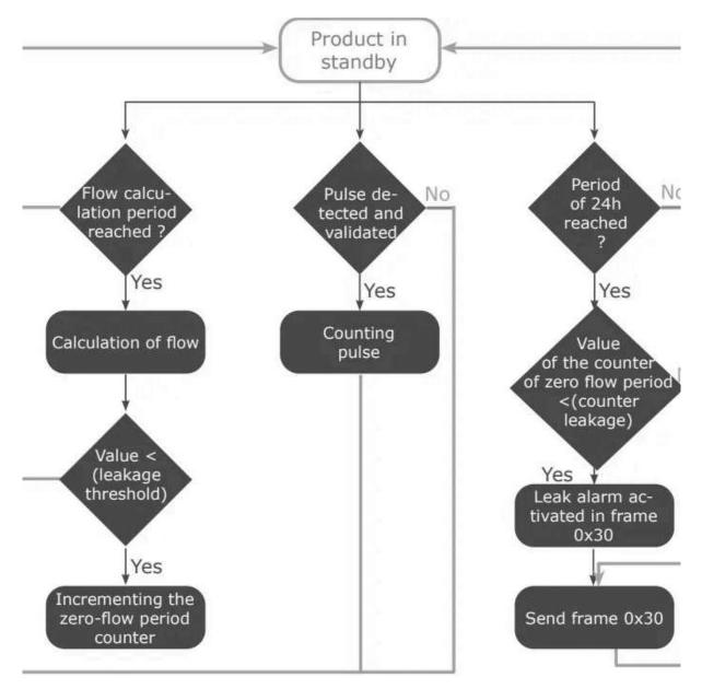
The flow rate corresponds to the number of pulses of the flow calculation period divided by the same period. It is expressed in pulses / hour.
