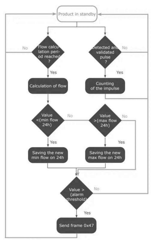
The flow rate corresponds to the number of pulses of the flow calculation period divided by the same period. It is expressed in pulses / hour.
