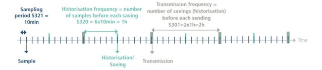
Procedure to follow to program its registers according to the chosen mode:
