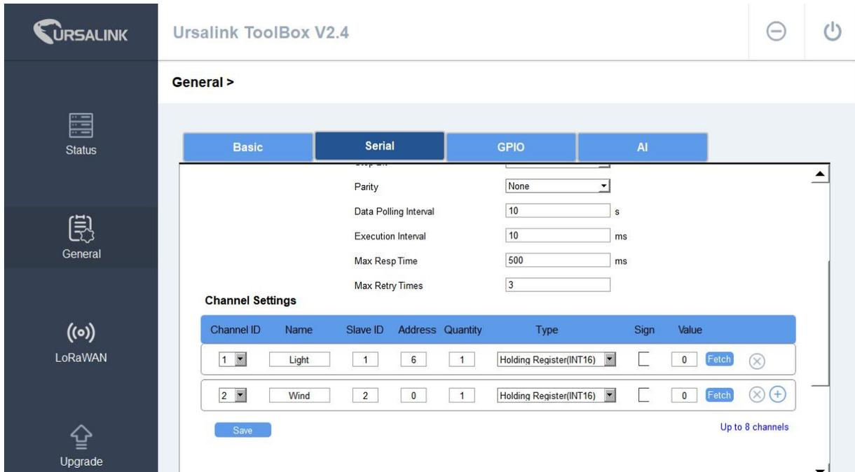
In this Quick Start Guide, UC11-N1 connects with two equipment (light sensor and wind speed sensor), both sensors use Modbus RS485.
