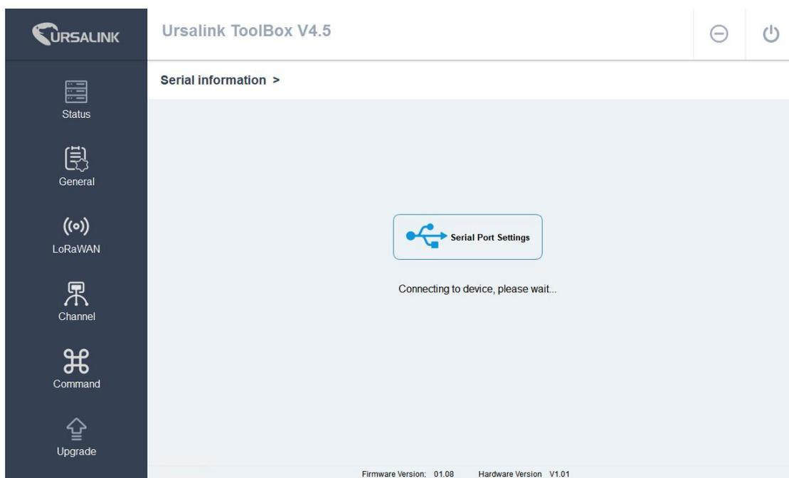
The software will display this interface when getting started. Here you can create a new setup, import an existing setup from your PC, or retrieve the current setup from UC1152.
