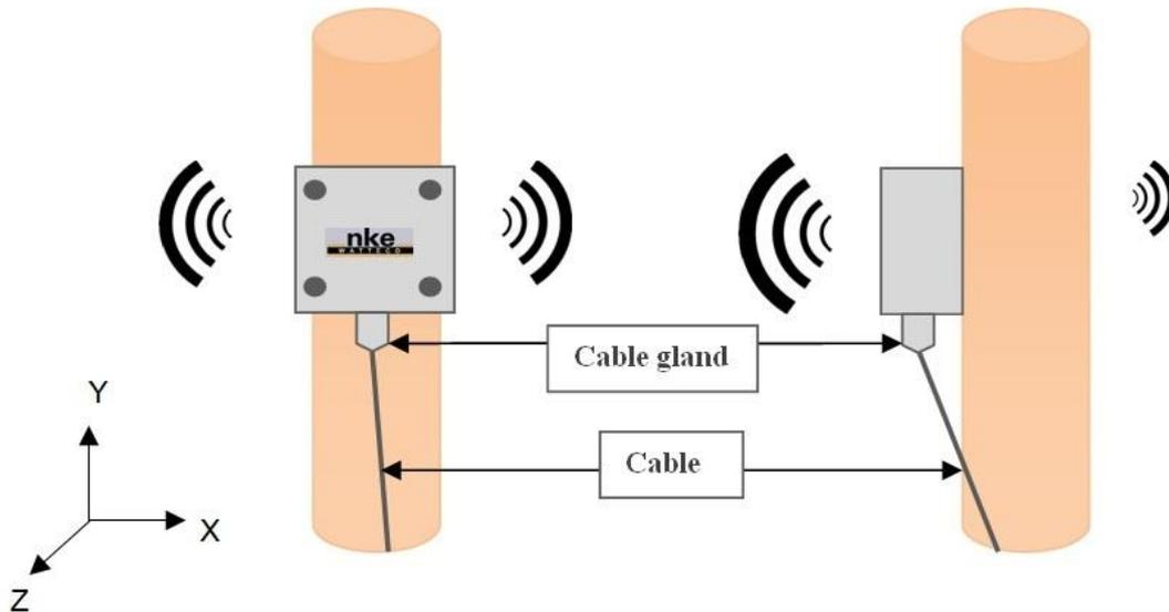
FIGURE 5 - BEST INSTALATION POSITION FOR THE MODBUS SENSOR
