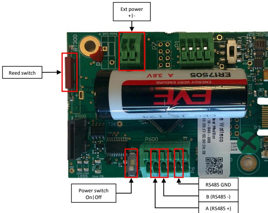
FIGURE 3 - AVAILABLE SIGNALS AND INTERACTION ON MODBUS SENSOR
