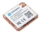
Dragino LA66 is a small wireless LoRaWAN module that offers a very compelling mix of long-range, low power consumption, and secure data transmission. It is designe quickly deploy industrial-level LoRaWAN and IoT solutions. It helps users to turn the idea into a practical application and make the Internet of Things a reality. It is easy to everywhere.
