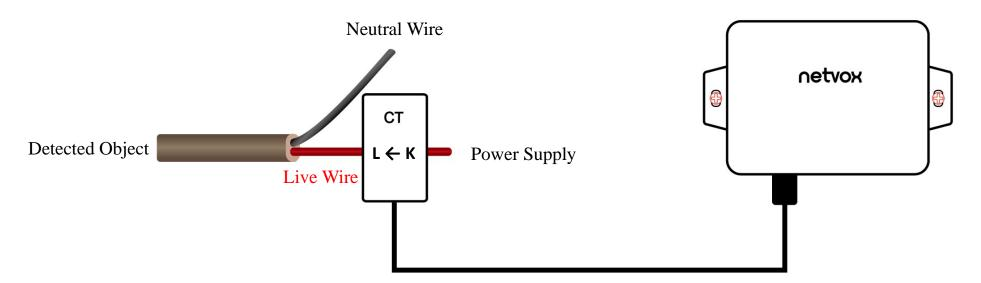
CT Wiring Schematic Diagram (Current direction  $K\rightarrow L$ )
