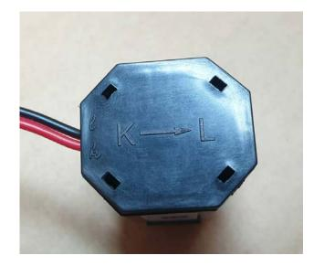
If the live wire and the neutral wire are connected together at the same time, they will offset each other and the measurement is 0.
