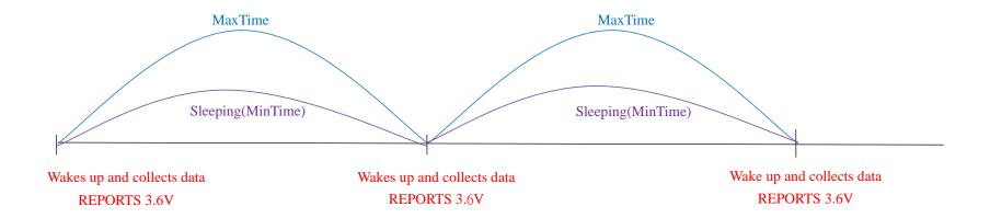
Note: MaxTime=MinTime. Data will only be report according to MaxTime (MinTime) duration regardless BatteryVoltageChange value. **Example#2** based on MinTime = 15 Minutes, MaxTime= 1 Hour, Reportable Change i.e. BatteryVoltageChange= 0.1V.
