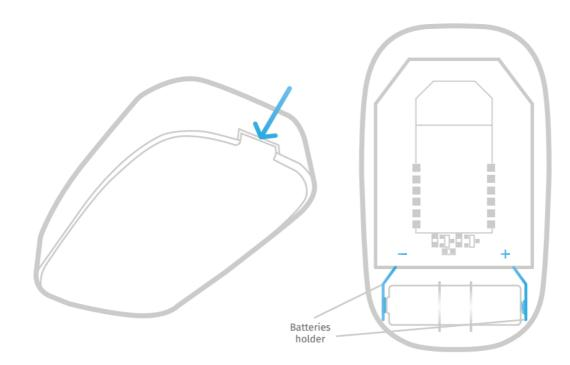
Disassembled MClimate Multipurpose Button LoRaWAN®, top view
