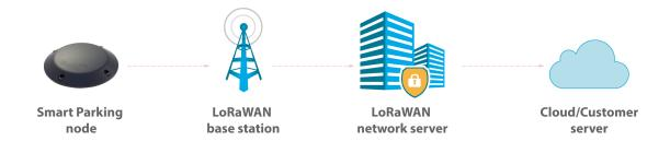
Figure: Simplified Smart Parking network architecture
