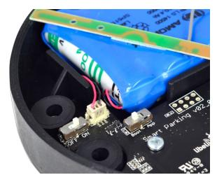
Figure: Smart Parking node "user switches"
