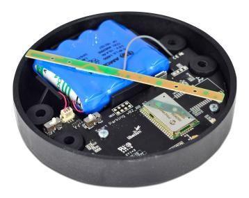
Figure: Base of a Smart Parking node
