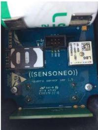
2. Put the cover back on. A sensor is now initialized and ready to be installed.
