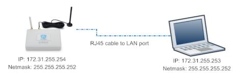
The LG308 has a fall-back ip in its LAN port. This IP is always enabled so user can use fall back ip to access LG308 no matter what the WiFi IP is. The fall back ip is useful for connect and debug the unit.
