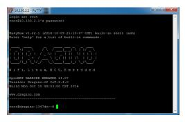
The "logread -f" command can be used to debug how system runs.
