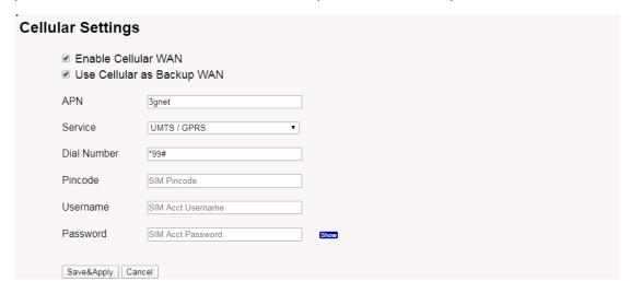
Note \*: For LG308 which doesn't have the cellular module, this page will shows Cellular not detected.
