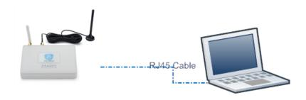
The LG308 <u>LAN port</u> is configured as DHCP router by default, user can connect the PC to LAN port and set PC to DHCP mode, it will get IP from LAN port and be able to access to the device. The default IP in LAN port is 10.130.1.1
