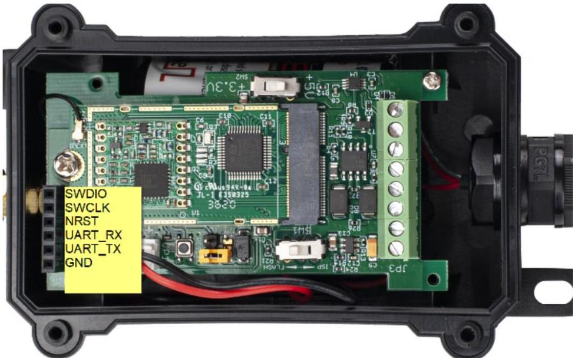
In the PC, you need to set the serial baud rate to **9600** to access the serial console for LSE01. LSE01 will output system info once power on as below:
