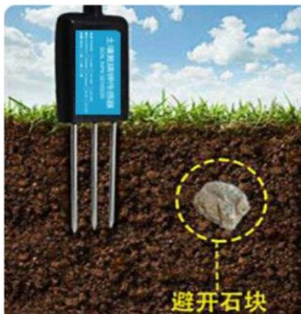
Choose the proper measuring position. Avoid the probe to touch rocks or hard things. Split the surface soil according to the measured deep. Keep the measured as original density. Vertical insert the probe into the soil to be measured. Make sure not shake when inserting.
