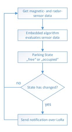
The sensors data are processed by the devices embedded algorithm. The algorithm output is the parking state "free" or "occupied". The device checks, if the parking status has been changed since the last processing run and in case the parking state change will be communicated via the LoRa interface. This means, that the parking sensor will only report, if the parking state has changed.
