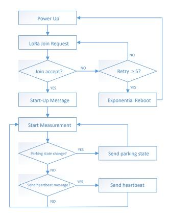
The parking state message can be configured as not confirmable. This reduces the use of duty cycle to acknowledge all messages, but may also reduce the percentage of successfully received messages by the Gateway.
