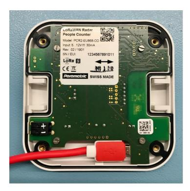
Connect the sensor to your Computer using a USB Cable.
