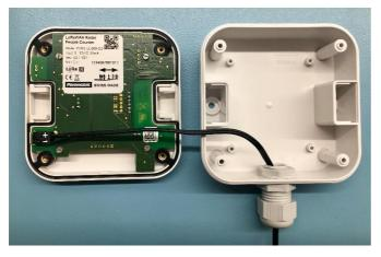
Guide the cable through the cable gland.
