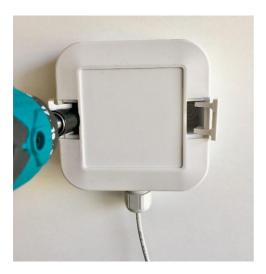
Ensure that the cable gland is fully tightened. Open the hatches on the front of the casing and drill two screws into the wall.
