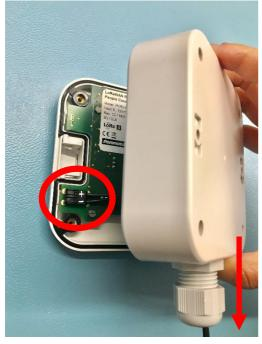
Before closing the casing, make sure that the two components are aligned as depicted:
