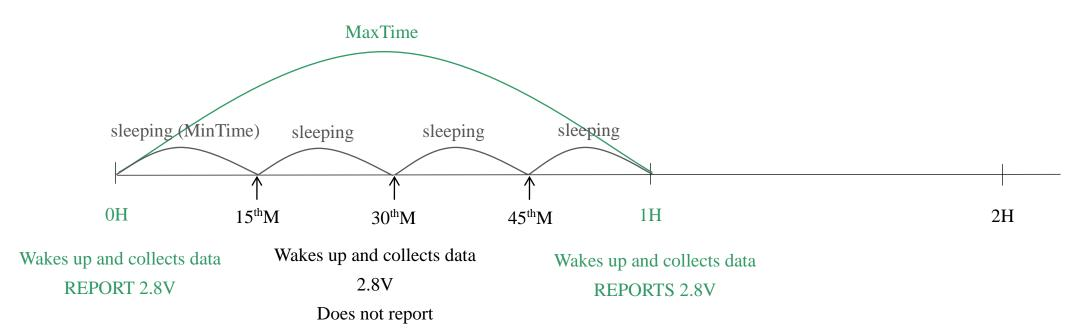
Example#3 based on MinTime = 15 Minutes, MaxTime= 1 Hour, Reportable Change i.e. BatteryVoltageChange= 0.1V.
