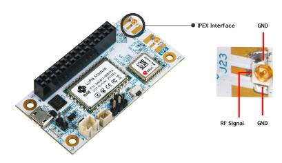
Figure 7: iPex Antenna Interface for LoRa Antenna
