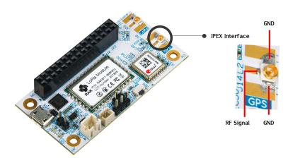
Figure 10: iPex Interface for GPS Antenna
