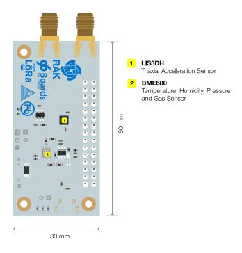
Figure 2: RAK5205 Dimension and Sensors Available
