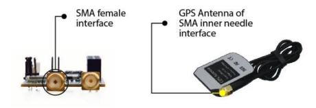
Figure 9: SMA Female Interface for GPS
