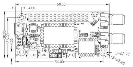
Figure 14: RAK5205 Detailed Dimensions
