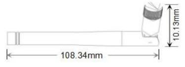
Figure 8: LoRa Antenna Dimension
