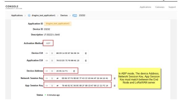
Note: user just need to make sure above three keys match, User can change either in TTN or Device to make then match. In TTN, NETSKEY and APPSKEY can be configured by user in setting page, but Device Addr is generated by TTN.
