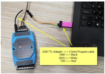
In PC, User needs to set **serial tool**(such as <u>putty</u>, SecureCRT) baud rate to **9600** to access to access serial console for LT. The AT commands are disable by default and need to enter password (default:**123456**) to active it. As shown below:
