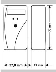
The EURISII electronic heat cost allocator comes in one-sensor and two-sensor versions. It is available with optical and/or radio interface. The radio protocol applied is the W-MBUS protocol according to DIN EN13757-4 in the T1 or S1 mode. The data to be transmitted can be coded using AES128 according to the OMS standard.
