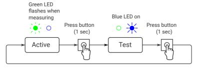
Illustration 3: Switching between active and test mode.
