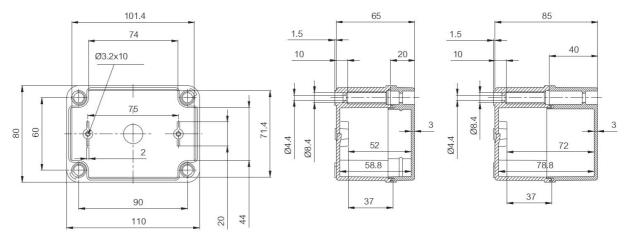
Illustration 6: Housing dimensions (in mm). Note: Drawing not including cable gland and sensor.
