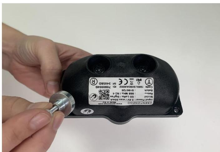
3. After initialization sensor starts to measure and logs into the network. Within 1 minute you should hear short beep 1 time. If the transmission is not complete you can hear short beep 2 times. In that case, you have to check whether the measurement was transferred to Sensoneo Waste Management System. Make sure you are in the coverage area of the network signal.
