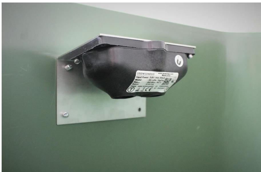
Please point the transmitter resonator (marked yellow) to the center of the bin. Do not point the sensor axis to the center. Pointing the transmitter to the center of the bin is important to achieve better measurement results, especially for smaller container sizes.
