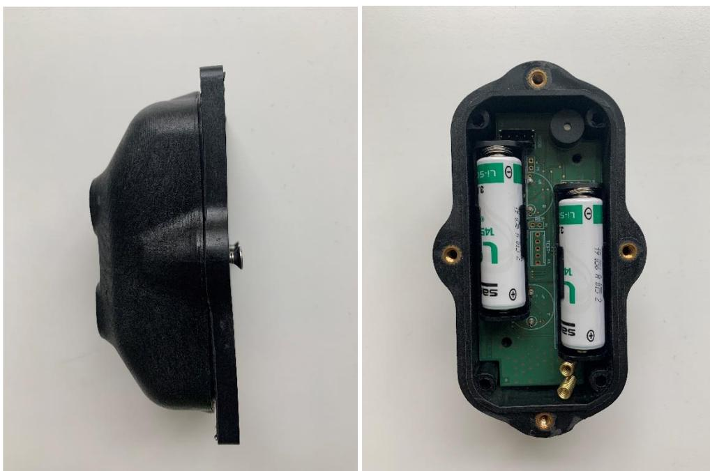
2. Attach the magnet to the sensor as shown in the picture (turn On/ Off ), you will hear the short beep 4 times.
